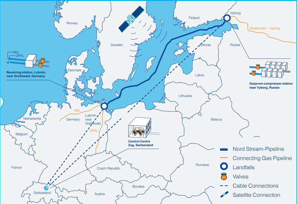
Nord Stream links the massive gas reserves in Western Siberia with the European gas distribution grid. The switching point of the project is the landfall facility in Lubmin, near Greifswald, Germany.
